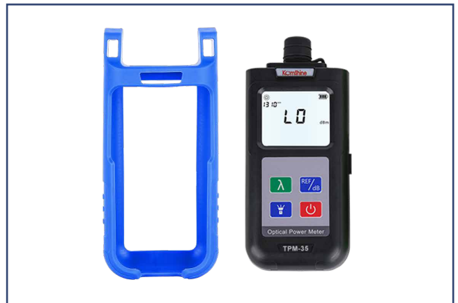
Split protective jacket
