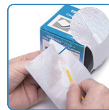
Wipe bare fiber directly
