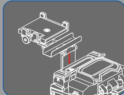
Insert the support frame into the socket of the base, adjust it to a proper height, and tighten the screws
