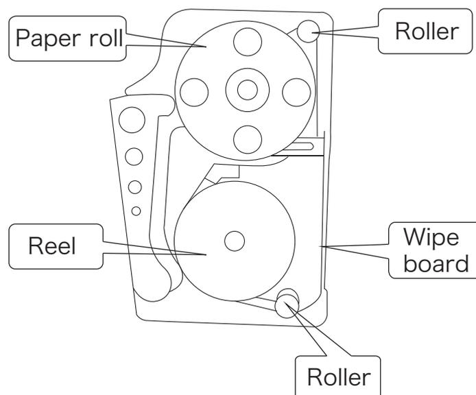
1. Use a coin or flat-head screwdriver to turn the screw, open the casing, and remove the roll paper tube and reel.
