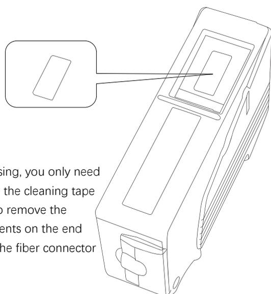
When using, you only need to swipe the cleaning tape gently to remove the attachments on the end face of the fiber connector ferrule.
