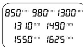
On the optical power meter interface, short press the "λ" key to switch the measurement wavelength, select 7 different test wavelengths, 850nm/980nm/1300nm/1310nm/1490nm/1550nm, 850nm, 1625nm to ensure the accuracy of the test, select the wavelength should be consistent with the wavelength of the measured optical signal.
